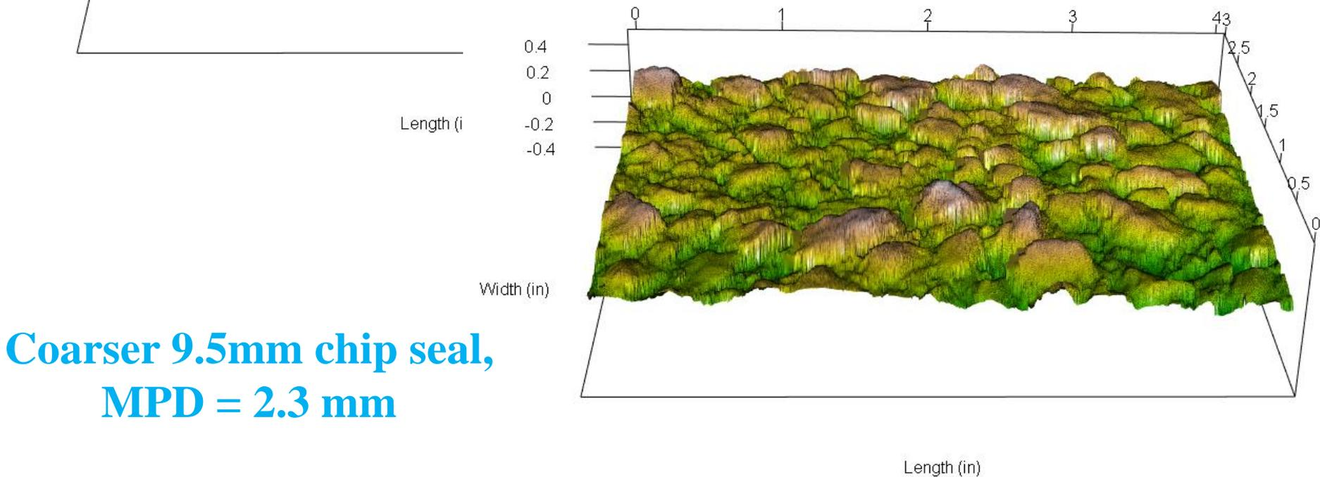
**Coarser 9.5mm chip seal,
