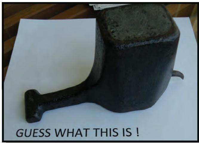
**Clay** has advised that the device is a lead spline weight that is used by draftsmen (when they actually used pens, pencils and paper) to hold a flexible curve in place while drawing or tracing a curved line. See photo below.
