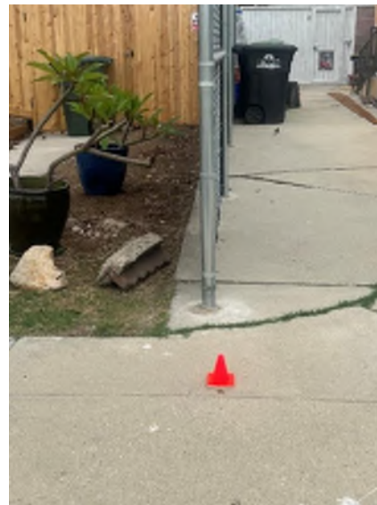
Above: A survey monument is in front of the orange cone. Notice that the fence was not constructed along the property line.
