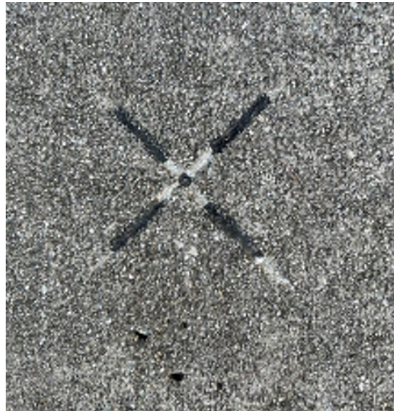
Above: A scribed cross used as a temporary reference during field work. Both this and the adjacent are evidence of survey. This cross is approximately 1.25 inches.
