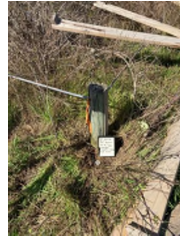
Figure 7: 5/8" rebar with 1-1/2" diameter aluminum cap monument near a fence corner.
