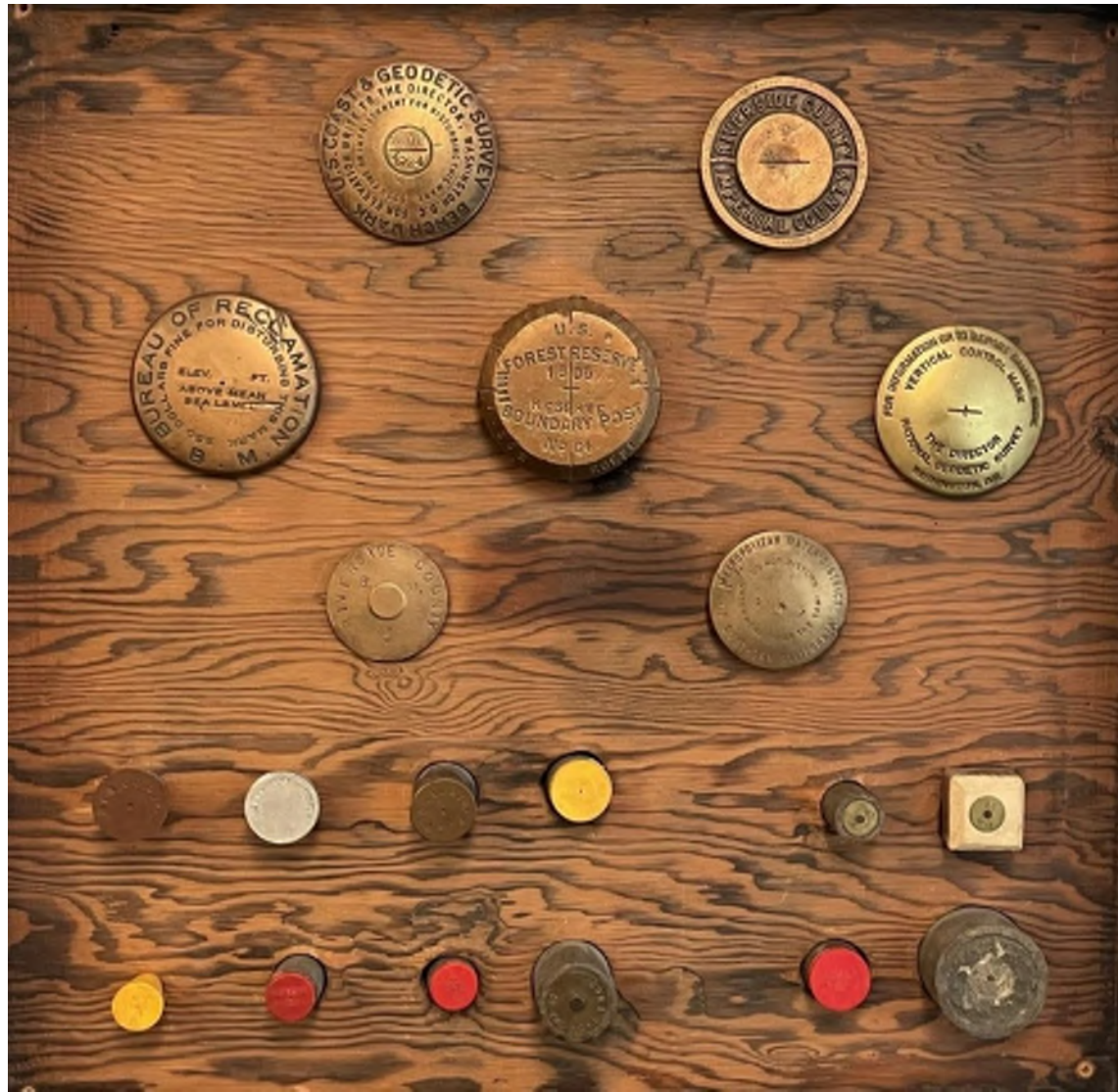
Figure 19: Examples of survey monuments on display at the County Surveyor’s office in Riverside County. For perspective, the large brass discs are 3 inches in diameter.
