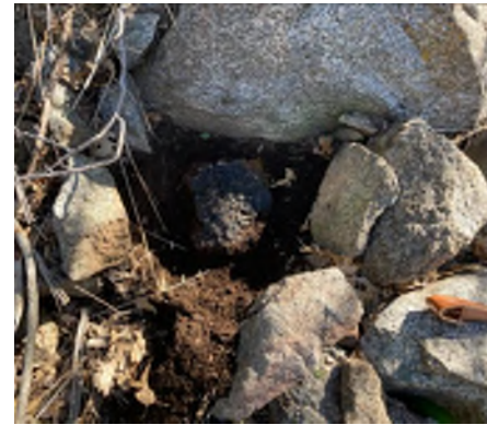
Figure 18: NWC Section 29, T9S, R1E, SBM burnt post in rock pile – original monument.
