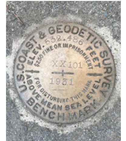
Figure 9: example of a 3" diameter brass benchmark set flush in concrete.
