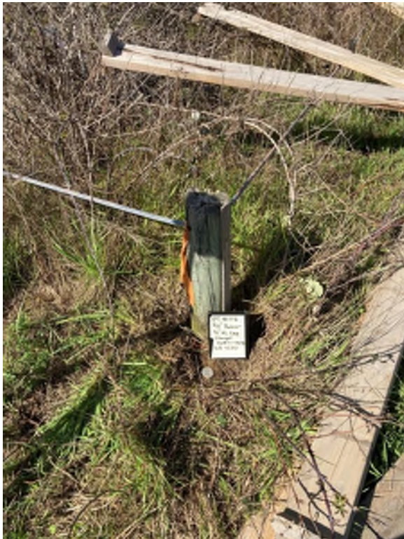
Above: 5/8" rebar with 1-1/2" diameter aluminum cap monument near a fence corner.
