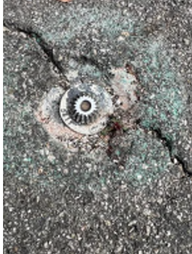
Above: A gear spike and washer set in asphalt. These spikes are hard and brittle so care must be used when driving them into hard surfaces as they can break leaving the broken shaft in place.
