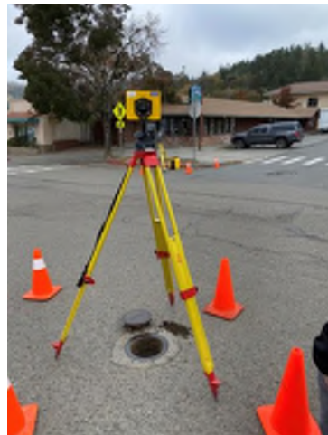
Figure 1: Survey equipment set up over a monument well. The lid is approximately 11.5 inches in diameter and stamped "monument".
