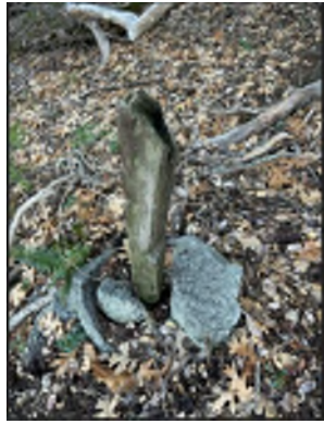
Figure 16: NWC Section 28, T9S, R1E, SBM original post in rock pile. See bearing tree in photo to the right.
