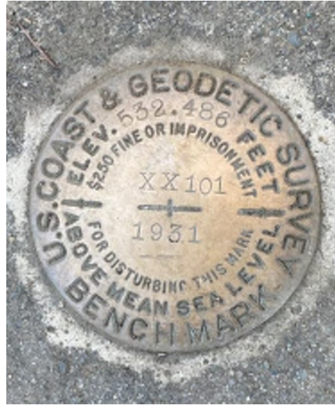
Above: Example of a 3" diameter brass benchmark set flush in concrete. Note the inscription "$250 fine or imprisonment for disturbing this mark".
