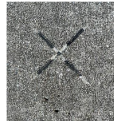
Figure 11: A scribed cross used as a temporary reference during field work. Both this and the adjacent are evidence of survey. This cross is approximately 1.25 inches.
